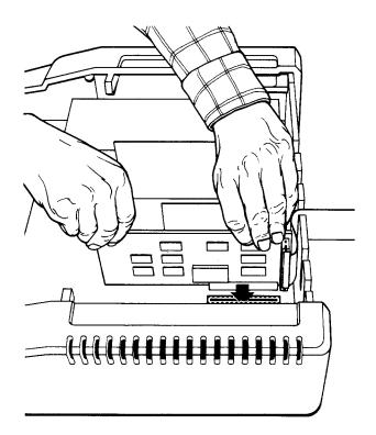
Install the floppy card in any slot according to the instructions that came with the computer.
