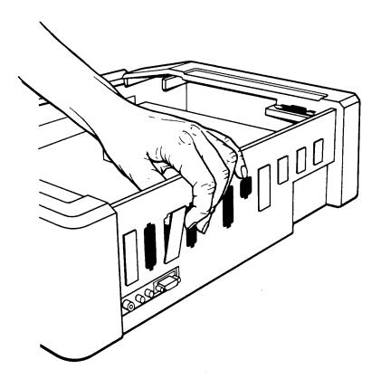
5. Plug the tap cable (OCS I) or drop cable (OCS II) into the interface card.
